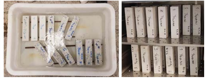
Fig. 5. Prismatic test samples (Series V) submerged (left), prismatic test samples in the stove (right) during the water-stove cycle.
